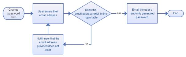
Figure 24: Flowchart of the change password process
