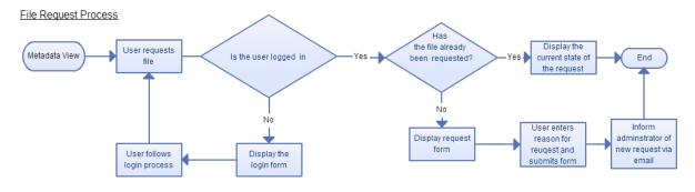
Figure 27: Flowchart of the file request process
